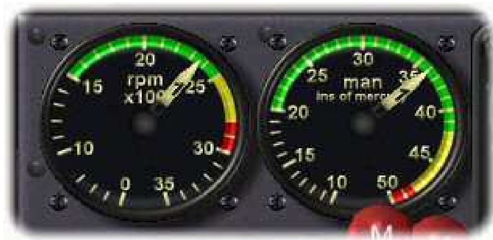
DC-3 Climb power settings: 2350 RPM, left, and 36 in. Manifold Pressure, right.
